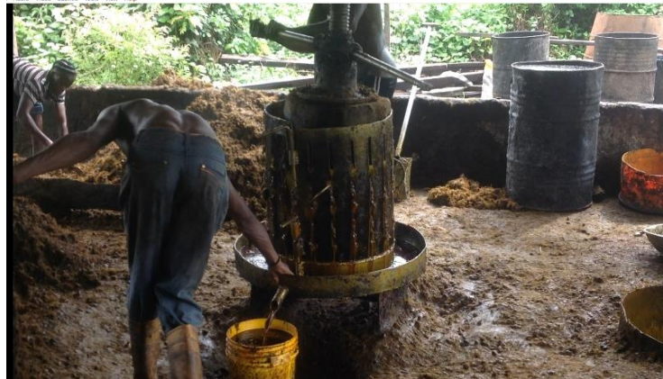
Traditional manual spindle method for oil extraction
